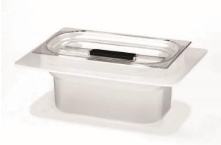
When cleaning with solutions that damage stainless steel, the ultrasonic tank can be protected by using an acid-resistant polypropylene tub. The ultrasonic energy is transferred from the liquid in the tank through the walls of the tub to clean items inside the tub. The tub hangs from the rim of the tank and comes with a transparent lid.
