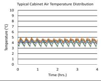
Performance data acquired at 22°C ambient, 4°C nominal set point in an empty cabinet with drawers using validation ballast probes, during stabilized steady state operation and a DAQ sampling rate of one measurement every 10 seconds
