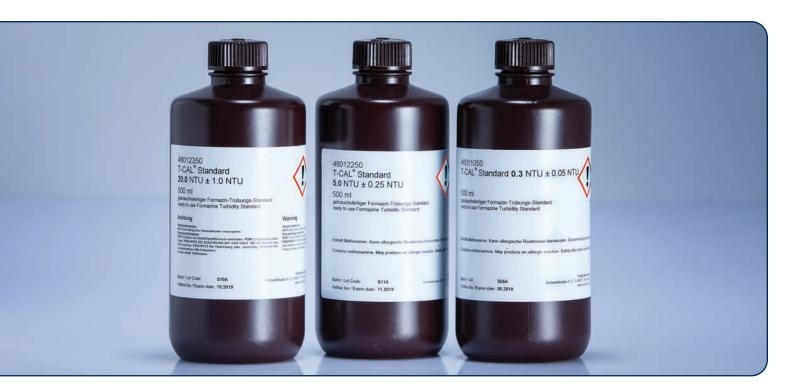
T-CAL® Turbidity Standard: A ready-to-use, stable Formazin standard that is prepared to a specific concentration, eliminates the opportunity or threat of preparation errors and is not susceptible to environmental variables.
