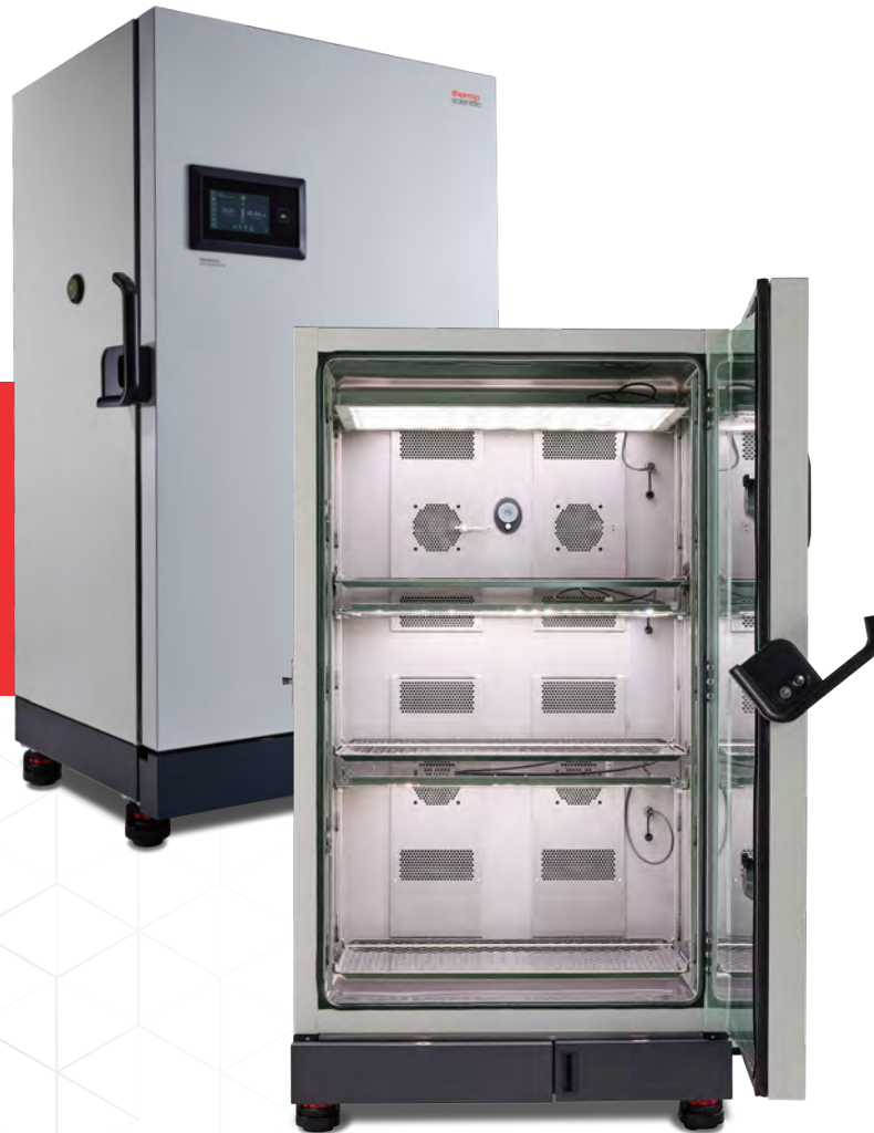
ELS750 with 3 plant growth LED modules installed.
