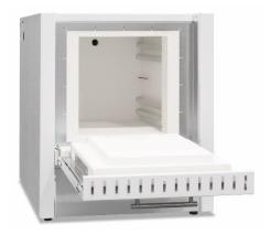
This furnace is only available with a flap door which can be used as work platform when loading or unloading. Fast heating times due to heating elements encased and protected in quartz glass tubes provide efficient heating. The combination of dual shell housing and superior insulation materials results in a very efficient power consumption.
