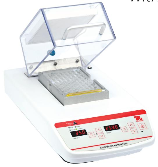
Multi-purpose Dry Block Heaters are ideal for applications that require temperature stability. The close tube-to-block contact enables maximum heat retention, resulting in efficient heating. High-wattage, constant-temp. Digital models offer exceptional temp. uniformity & stability for applications that require repeatable results. Units hold optional interchangeable modular blocks with over 40 options.
