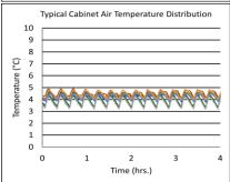
Performance data acquired at 22°C ambient, 4°C nominal set point in an empty cabinet with drawers using validation ballast probes, during stabilized steady state operation and a DAQ sampling rate of one measurement every 10 seconds
