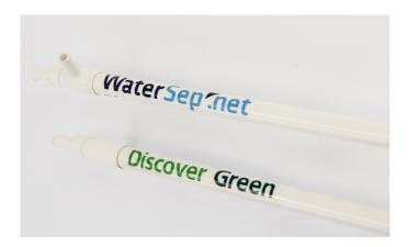
The Discover Green hollow fiber membrane cartridges are the cartridges of choice for small scale preparative protein and virus concentration/diafiltration, and cell clarification applications for volumes that range from 50 ml to 400 ml. The Discover24 Green cartridges have a membrane surface area of 107 cm², providing a typical permeate flow rate of 32-64 ml/hr for ultrafiltration applications and 21-43 ml/hr for microfiltration applications.
