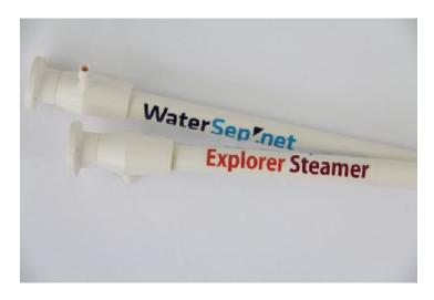
The Explorer41 Steamer is a small to laboratory-sized autoclavable, gamma irradiated, re-usable hollow fiber cartridge made with WaterSep's low binding, glycerin free modifed PES membrane (m-PES) which provides a process flux and product recovery that exceeds other crossflow devices. Explorer41 Steamer cartridges are ready to use without any pre-rinse or sanitization, or can be autoclaved as is, or in an assembly.
