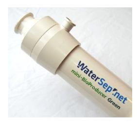
The mini-BioProducer Green hollow fiber cartridges are designed for pilot and production scale production and are the perfect tools for process development. With a surface area of 1.30 m², the mini-BioProducer24 Green HF cartridge can accommodate batch volumes between 10L and 100L with a typical permeate flow rate of 39 to 78 L/hr for ultrafiltration applications and 26 to 52 L/hr for microfiltration applications.
