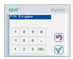
**PIN** for enhanced security. The unit can be configured with a PIN inquiry function to protect against accessing by unauthorised persons or for enabling only selected functions.
