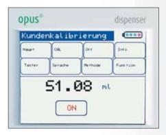
■ enables you to access the selection menu. Calibration, operating language selection, activation of the method memory? A further push of the button and you can access the respective configuration menu
