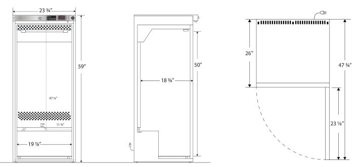
Note: This unit must have 4" clearance on sides and back for adequate ventilation
