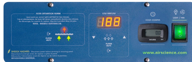
FSA/Autocal Control Panel
