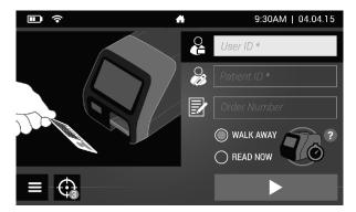
2. Input the Patient ID and Order #, if applicable, using the barcode scanner or manually enter the data using the on-screen key pad.
