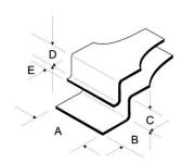
**Tip dimensions (Wafer tweezers):** A (tip width) 6.5 mm – 0.256 inch
