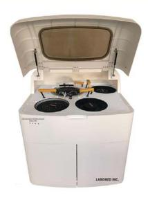
Laborned introduces an automatic biochemistry analyzer with varying testing capacities. FACA-601 conducts 600 tests/hr with True Random Access .
