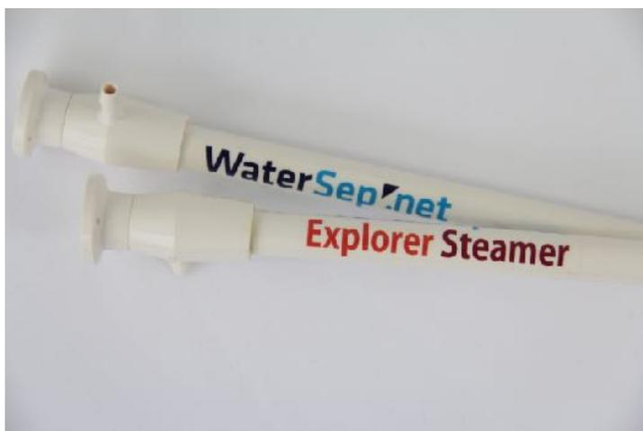
The **Explorer24 Steamer** is a small to laboratory-sized autoclavable, gamma irradiated, re-usable hollow fiber cartridge made with WaterSep's low binding, glycerin free modified PES membrane (m-PES) which provides a process flux and product recovery that exceeds other crossflow devices. **Explorer24 Steamer** cartridges are ready to use without any pre-rinse or sanitization, or can be autoclaved as is, or in an assembly.
