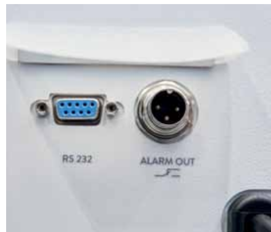
Standard-issue RS 232 interface and alarm contact
