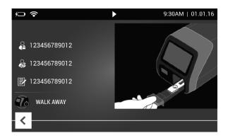
4. Insert the prepared Test Cassette into the drawer of Sofia 2 and close the drawer.
