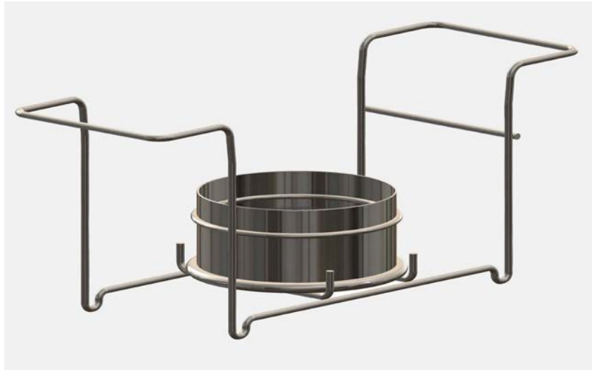
Illustration 4.9.2.1. Sieve holder with laboratory sieve 100 mm
