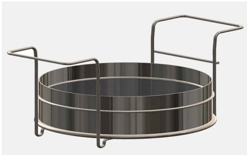
Illustration 4.9.2.2. Sieve holder with laboratory sieve 200 mm
