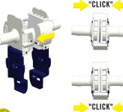
Align the connector halves with the pull tabs hanging down. Slide the two halves together. Independently squeeze each side of the connector until you hear an audible "CPC Click."
