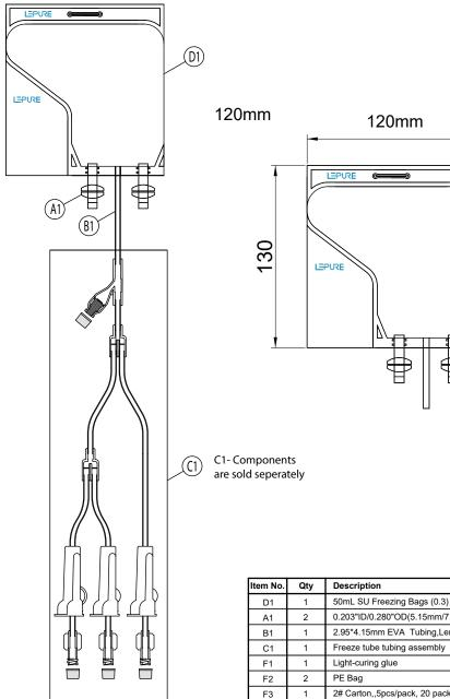
Note: labeling is forbidden on the Freezing Bags body; a small label can be placed on the surface of the inner PE bag and a product label on the outer PE bag
