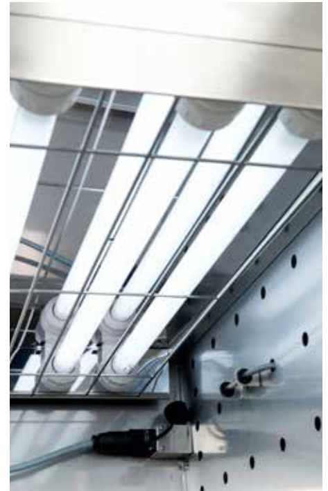
Interior of Forma Vertical Light Chamber with animal hatching light modules installed.
