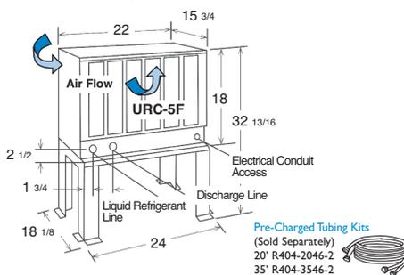
Voltage supply for the URC Remote Condenser is supplied from the Ice Maker. No additional circuit is required.
