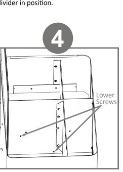
Keeping the rounded corner at the top left, reposition divider at a slanted position, resting on lower screws.
