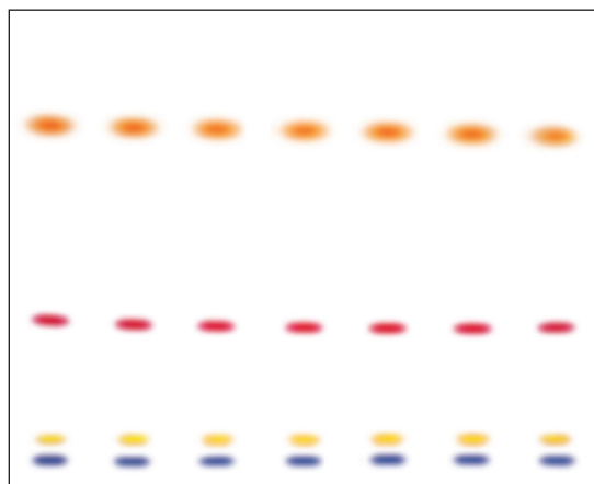
Ph Eur performance test on EMD Millipore TLC silica gel 60G plate
