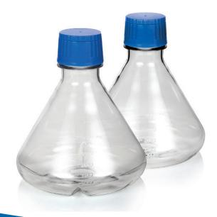
TriForest Fernbach culture flasks are sterile and designed for single use, however, it can be autoclaved and reused multiple times. They are ideal for all shaker/suspension culture. Like all TriForest Erlenmeyer flasks, the 3L Fernbach flasks come with the patented DuoCAP®. They are certified pyrogen and nuclease free. These flasks are available with or without baffles and are a complementary addition to TriForest Erlenmeyer Family.
