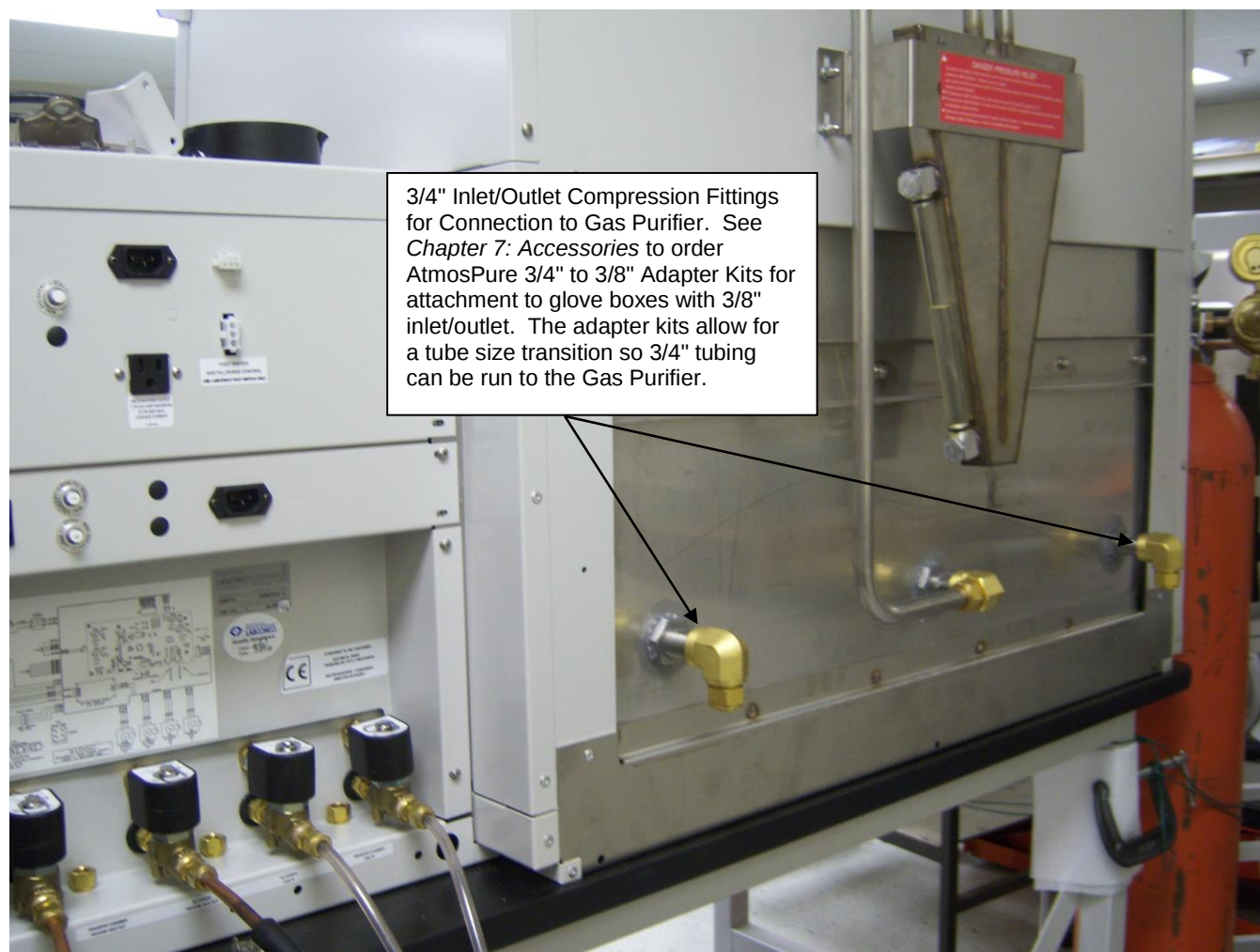
Figure 3-2 Typical Plumbing Connection for the Circulation Lines
