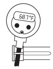
Insert the probe into the "loop" on the cover. It makes a perfect holder.
