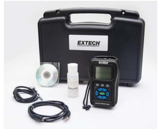
All models include 2oz bottle of couplant, 2 AA batteries, Transducer (5MHz, 0.375" diameter ) with potted cable, and hard case. TKG150 and TKG250 also include protective holster, Echo to Echo, B-Scan, USB cable, and Extech XPorter software.
