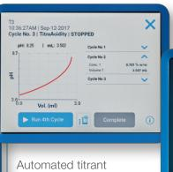
delivery system with high-accuracy burette and dispenser provides consistent results and automatic results calculations simplifies analysis and reduces computational errors.
