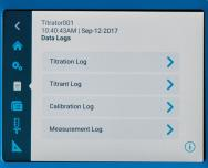
Internal data storage maintains a history of sample titrations, titrant standardizations, electrode calibrations and direct measurements – all with date and time stamp – to preserve critical data and facilitate easy data transfer to an external device.
