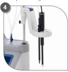
Bottle holder helps secure titrant to prevent spills and can be easily disconnected from the titrator for flexible placement on the lab bench.
