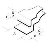
**Tip dimensions (Wafer tweezers)**: A (tip width) 9.5 mm – 0.374 inch
