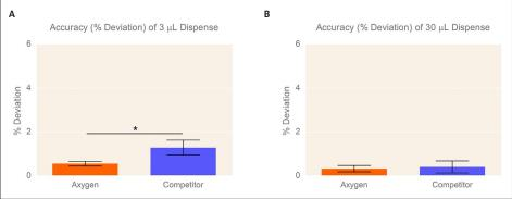
Figure 2. Accuracy (% D) analysis of 384-well 30 µL tips. The % D of Axygen and Competitor 30 μL tips dispensing (A) 3 μL and (B) 30 μL volume using the Biomek FX liquid handler was determined using the Artel MVS System. (A) Axygen tips displayed significantly lower % D and, thus, higher accuracy than Competitor tips dispensing 3 μL. \*P<0.05. (B) There was no significant difference in % D between each brand dispensing 30 µL. Data shown with SD for 3 independent experiments of 384 wells each.
