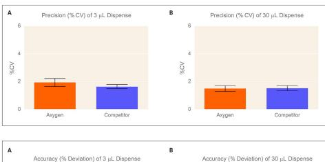
Figure 1. Precision (% CV) analysis of 384-well 30 µL tips. The % CV of Axygen and Competitor 30  $\mu L$  tips dispensing (A) 3  $\mu L$  and (B) 30  $\mu L$ volume using the Biomek FX liquid handler was determined using the Artel MVS System. There was no significant difference in % CV between each brand. Data shown with standard deviation (SD) for 3 independent experiments of 384 wells each.
