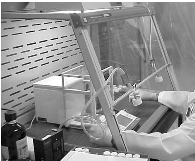
SafeBridge Consultants tested a 3' XPert Balance Enclosure's ability to contain airborne powders and found personal exposure to airborne concentrations of naproxen sodium was 25 ng/m 3 .
