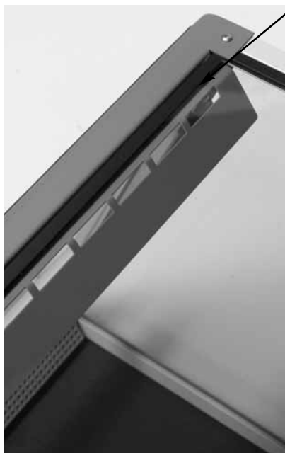
View from the top of the XPert Balance Enclosure showing the upper dilution air supply openings
