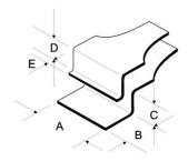
**Tip dimensions (Wafer tweezers):** A (tip width) 28.5 mm – 1.122 inch
