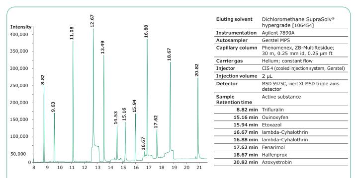
**Figure 7** Sample chromatogram (TIC), apple juice spiked. Sample preparation via liquid-liquid-extraction with EXtrelut® NT 20. Eluting solvent: Dichloromethane SupraSolv® hypergrade (1.06454.1000).
