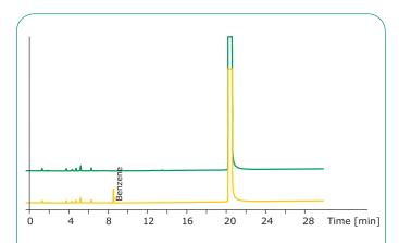
**Figure 4** Chromatogram of DMSO Headspace SupraSolv® 101900 without addition compared to a chromatogram of DMSO Headspace SupraSolv® 101900 with 0.8 ppm benzene.
