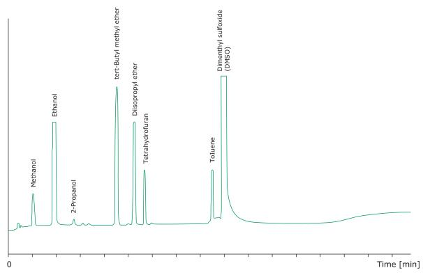
Figure 6 Quantification of residual solvents in an AFI using Dimethyl sulfoxide (DMSO) SupraSolv $^{\otimes}$  for headspace gas chromatography (101900).
