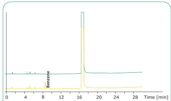
**Figure 5** Chromatogram of DMF Headspace SupraSolv® 100202 without addition compared to a chromatogram of DMF Headspace SupraSolv® 100202 with 0.8 ppm benzene.
