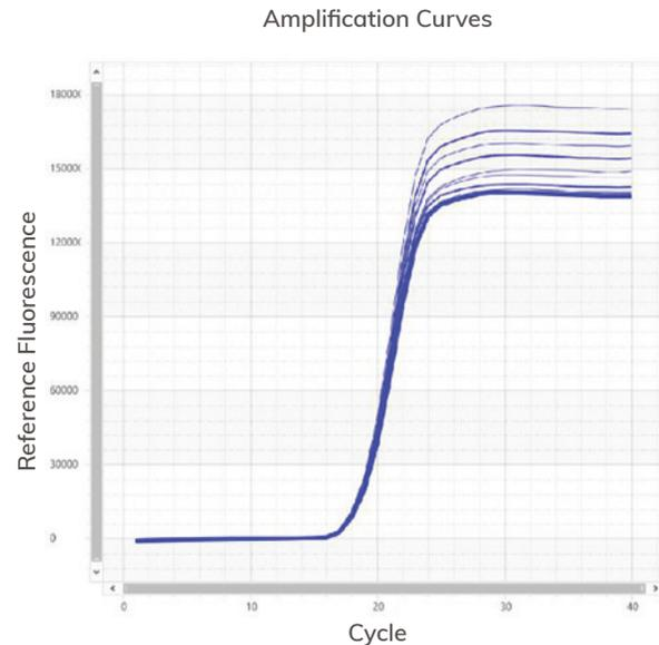
Optical design eliminates need for ROX. Amplification curves generated using human genomic DNA template along with human GAPDH primers and a no ROX SYBR Green qPCR mix.
