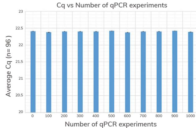
Robust design. After sequential sets of 1000 continuous qPCR experiments, a GAPDH qPCR assay was performed and Cq values were recorded at every 100 experiments points. Average Cq in each assay = 22.4,  $\pm 0.01$ .
