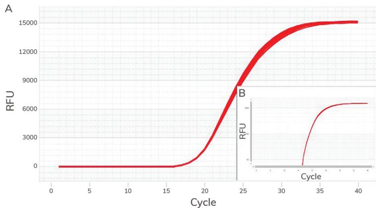
Unparalleled uniformity. Amplification curves for 96 replicates shown on a linear plot (A) and a logarithmic plot (Figure B). In each well,  $10^5$  copies of GAPDH template were amplified in the presence of GAPDH primers and BioRad™ Sso Advanced SYBR Green Mix®. Average Cq = 19.1, Coefficient of variance (Cv)= 0.002.
