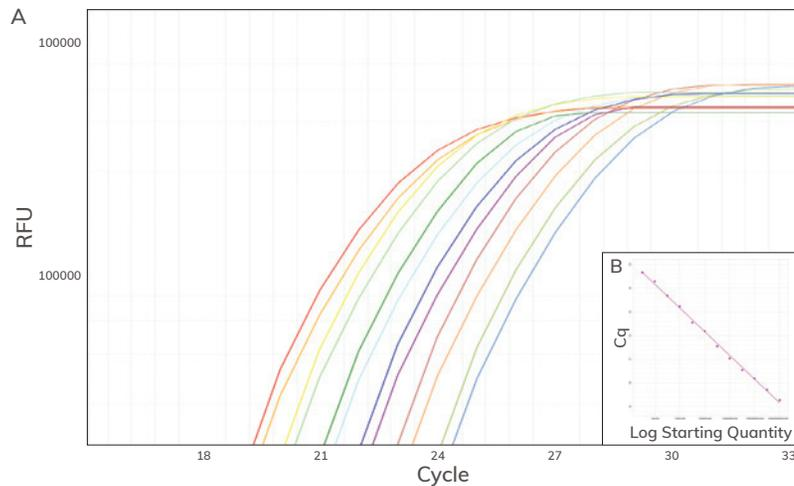
Reliable detection of 1.5-fold differences. Figure A. Amplification curves for assays of GAPDH in a dilution series of human reference cDNA (n=3). Assays were conducted using BioRad™ Sso Advanced SYBR Green Mix®. Figure B shows the standard curve obtained by plotting Cq values vs the amount of template DNA (copies/μl). R<sup>2</sup>=0.998, efficiency = 99.89%.
