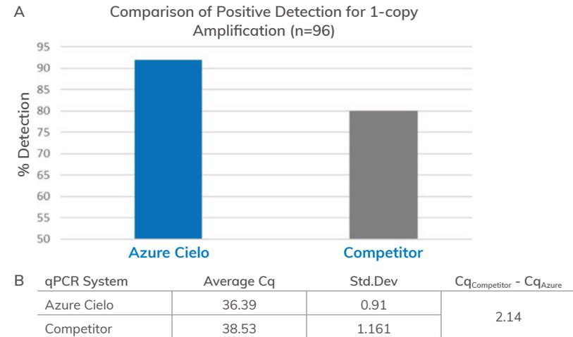
Superior single copy detection. Real-Time PCR was carried out using BioRad Prime PCR Probe Assay for GAPDH, 1 copy of Human Reference GAPDH DNA Template and Biorad Multiplex Supermix. A) Comparison of amplification detection in Azure Cielo Real-Time PCR system and Competitor shows higher rate of 1-copy detections. B) Average Cq obtained from Azure Cielo System is 2 cycles earlier than Competitor. Cqs from the above experiment were averaged.
