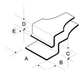
**Tip dimensions (Wafer tweezers):** A (tip width) 12.0 mm – 0.472 inch
