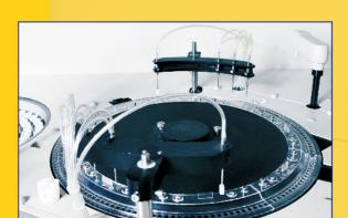
■ Eight channels washing station for each cuvette cleaning, automatic record and deduct cuvette blank value. Heavy washing function available for "dirt cuvette" to ensure each cuvette perfectly clean.
