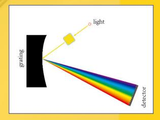
High resolution concave grating system, wavelength range 340-800nm, multi-wavelength polychromatic assay at the same time.
