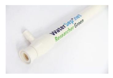
The Researcher Green crossflow hollow fiber membrane cartridges are designed for pilot scale and small scale production. It is the perfect tool for process development. With a surface area of 940 cm², the Researcher24 Green can accommodate batch volumes that range from 700 ml to 4,000 ml with a typical permeate flow rate of 2.8 to 5.6 L/hr for ultrafiltration applications and 1.9 to 3.8 L/hr for microfiltration applications.
