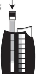
8 Insert test tube into Octa-Slide 2 Viewer.
