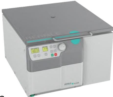
The Oil-Test Centrifuge OLEUM from HERMLE has a four place swing out rotor which accomodates cushions for oil test tubes according to ASTM: Conical or Pearshaped form! This purpose made unit has a normal air cooling without a heating or refrigeration system.
