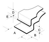
**Tip dimensions (Wafer tweezers):** A (tip width) 16.0 mm – 0.630 inch
