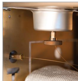
**Figure 5:** A correctly installed plate insert should be flush with the edge of the oven.
