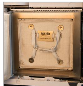
**Figure 6:** Only remove the plate insert once the system has sufficiently cooled.
