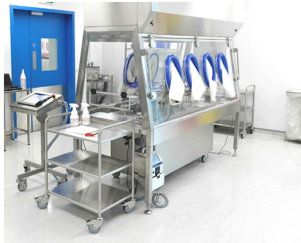
An isolator situated in a cleanroom
