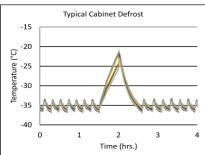
Performance data acquired at 22°C ambient, 4°C nominal set point in an empty cabinet with drawers using validation ballast probes, during stabilized steady state operation and a DAQ sampling rate of one measurement every 10 seconds
