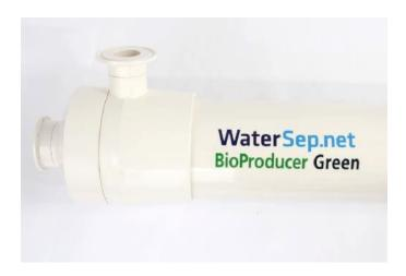
The BioProducer Green single use production scale hollow fiber cartridges are designed for biopharmaceutical concentration/diafiltration and clarification unit operations. With a surface area of 2.7 m², the BioProducer24 Green HF cartridge can accommodate batch volumes between 50L and 250L with a typical permeate flow rate of 81-162 L/hr for ultrafiltration applications and 54-108 L/hr for microfiltration applications.
