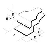
**Tip dimensions (Wafer tweezers)**: A (tip width) 20.0 mm – 0.787 inch
