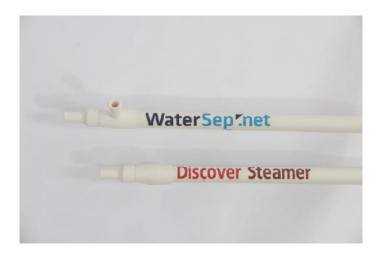
The Discover24 Steamer is a small scale autoclavable, gamma irradiated, re-usable hollow fiber cartridge, made with WaterSep's low binding, glycerin free modifed PES membrane. The Discover24 Steamer is ready to use without any pre-rinse or sanitization, or can be autoclaved as is, or in an assembly.
