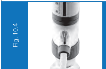
Before using the instrument, turn the valve to 'Dispensing'. (Fig. 10.4)
