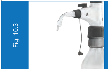
Remove cap from the discharge tube. (Fig. 10.3)
