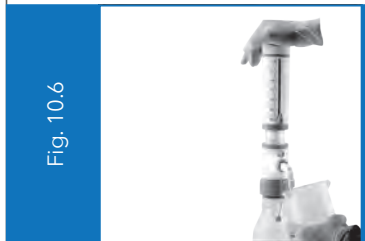
Gently lift the piston until the upper end. Press the piston downwards slowly and steadily with minimal force until the lower end. (Fig. 10.6)
